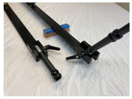
Posi-Lock Dips on both Cheek Blocks hold Gathering Arms securely in position when Adjustable Position (AP) Handle is tightened.
