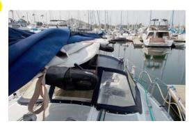
Zepp Sticks' ends wrapped with guards to protect mainsail cover. The guards depicted here are repurposed wind surf boom bras. Sail ties secure mainsail to Zepp Sticks' Bases before mainsail is covered. This full cover is also used in Zepp Sticks' sun shade configuration, with no "leaves" needed.
