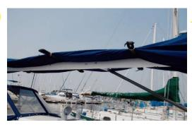
Gathering Arms removed and mainsail cover tucked in between Zepp Sticks' Base and mainsail In this position it is recommended Sunbrella "socks" be fitted on the exposed Zepp Sticks' ends to reduce effects of UV on composites.
