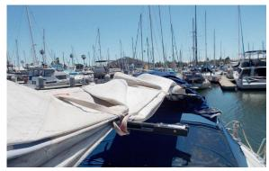
Gathering Arms removed and sail ties used to secure mainsail to boom. Zepp Sticks also provide a convenient platform for working on or folding and removing your good racing mainsail.
