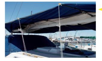
On this boat, a 4th Zepp Stick could be added to extend sun shade aft over the cockpit. You could also have your canvas shop make "leaves," akin to expanding a dining room table, that fasten to outboard sides of the splayed traditional mainsail cover.
