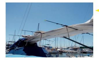
Zepp Sticks pictured have a Base length of 4 feet and in this configuration extend to a length of 8 feet.
